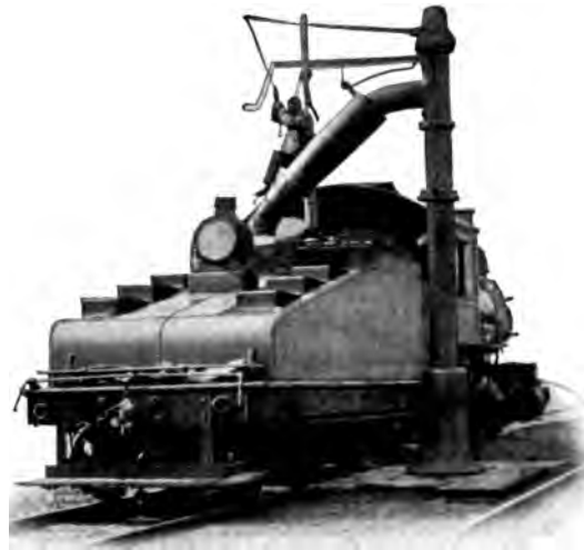
Low Tender—Man Hole 7 Feet Over Rail
